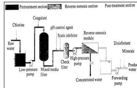
The permeate water produced from the RO membranes shall be collected in water tanks with booster pump, where blending quantity of other brackish water may added to the system before distribution. The final Chloride concentration will not be greater than 250mg/L. Post treatment to control PH and chlorine water disinfection shall be maintained before sending the water to the distribution network by the booster pump
